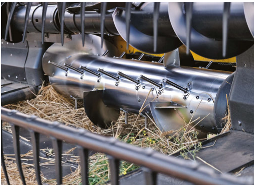
TYPHOON... The Typhoon Feed Drum's retractable fingers, aggressive pattern and smaller diameter barrel improve capacity and provide a better feed experience.
