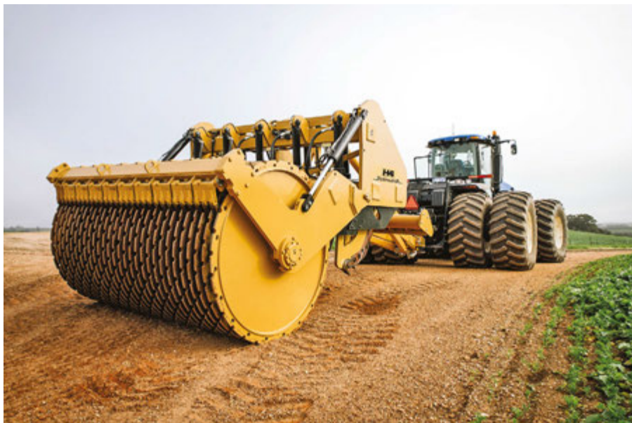
ALL TERRAINS... The Rocks Gone H4 Reefinator can crush between 500 and 3000 cubic metres per hour.
