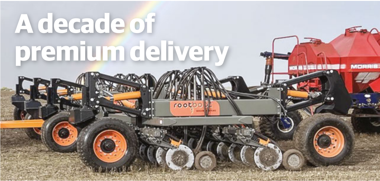
DELIVERY... The award-winning Rootboot places fertiliser and liquid product between paired seed rows with a buffer zone of soil between the seed and fertiliser.
